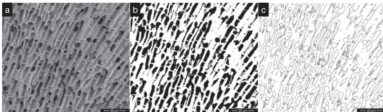
FIG. 2. Image conversion for determination of fraction calcified tissue. (a) Original scanning electron microscope photograph, (b) black and white threshold image, and (c) cartoon with pore spaces outlined. A cross-sectional view of sample A5 is shown in this example.
