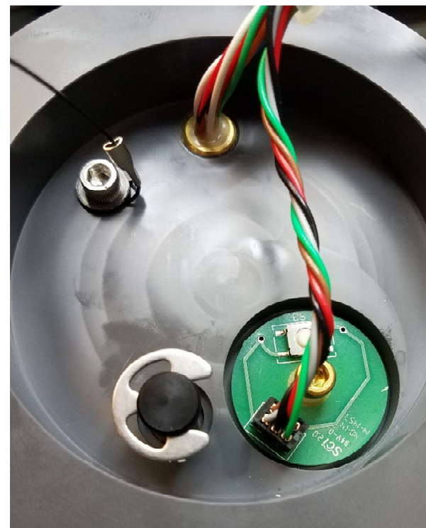
Figure 36 - Top Endcap Cable Assembly, 5-Pin Connector
